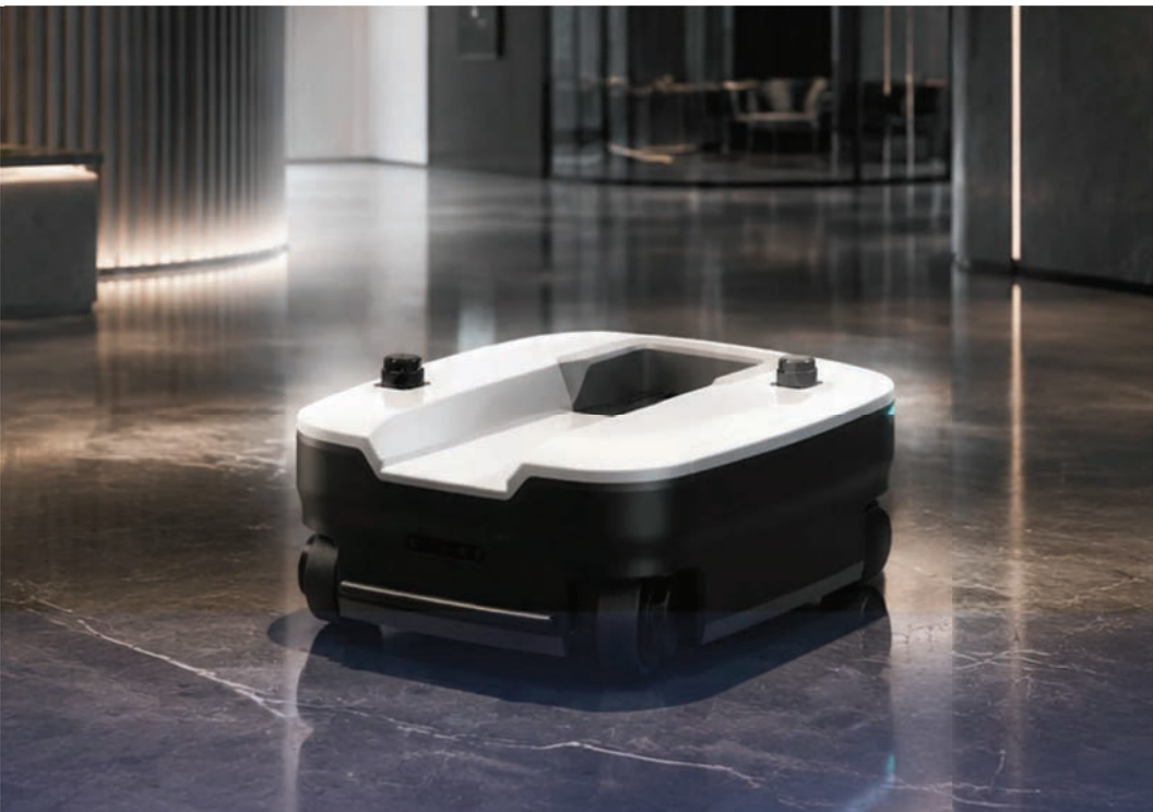
Mobile Base - Four-Wheel Steering & Drive
